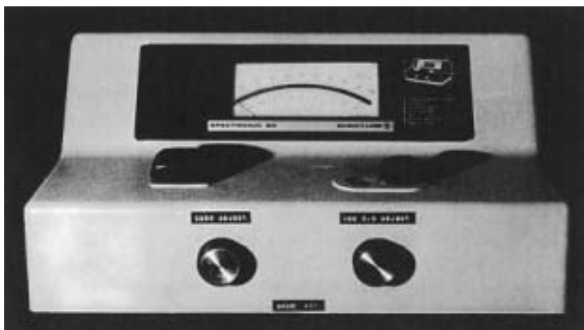
Figure IV.6 A Spectronic 20 spectrophotometer. The absorbance of a solution can be read to about 1%. (Sherman Schultz)
