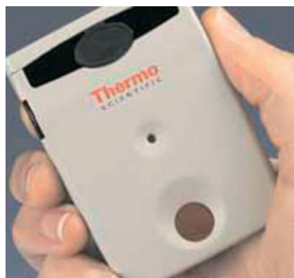
Figure 14 Electronic personal dosimeter from Thermo Scientific (NB: this is not an endorsement of any specific product or manufacturer; for illustrative purposes only!). (Reproduced with permission from Thermo Scientific 2009.)
