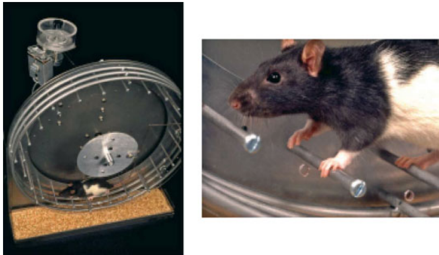
Figure 4 Apparatus used to study reward value of wheel-running. Pressing a lever on the wall a required number of times (a fixed ratio) releases a brake, and allows the rat to run for a specified number of seconds. (Reproduced with permission from Markowski et al. , 2002. © National Institute of Environmental Health Sciences.)
