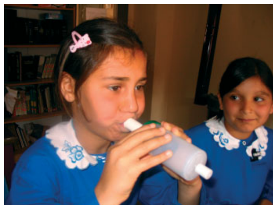
Figure 2 Exposure to benzene can be investigated using breath analysis. End-exhaled air was collected by children attending primary school in Turkey. The volatile organic solvents are transferred to a solid phase by the investigator directly after sample collection. In this way the organic compounds are well preserved for later analysis. (Reproduced with permission from J. Konings.)
