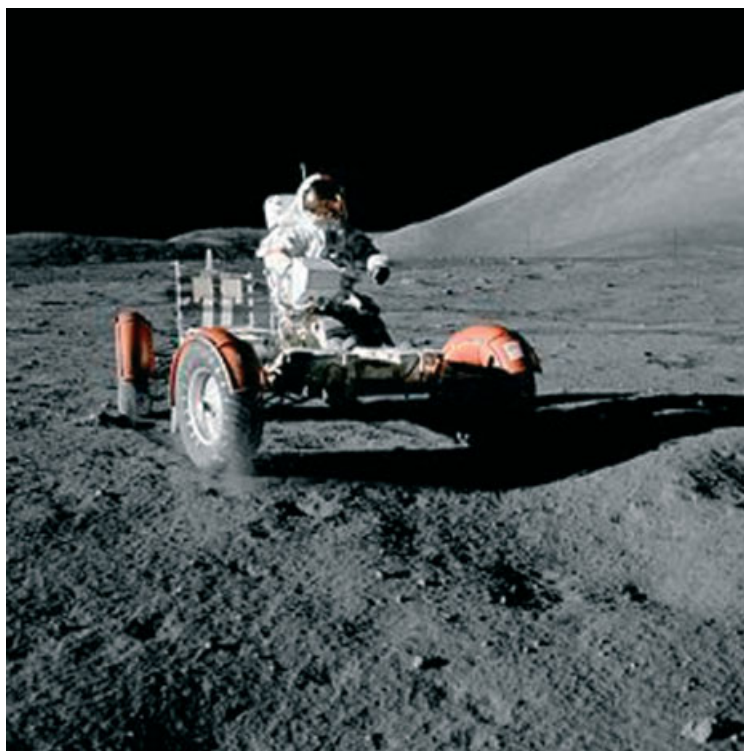
Figure 4 Apollo astronaut exploring the lunar surface during the Apollo missions. The open design contributed to lunar dust contamination of the suits of the astronauts. The main sources of lunar dust contamination came from exploration on foot and taking lunar samples. (Reproduced from NASA.)
