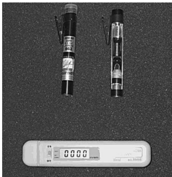
Figure 12 Direct-reading dosimeters. At the top are 'pen' or 'pencil' or 'pocket' dosimeters from which photon doses can be read directly by looking through the device to see a reading of dose to the dosimeter. At the bottom is a digital direct-reading dosimeter. (Reproduced from Christensen 2008a; 2008b, with permission from Radiation Emergency Assistance Center/Training Site (REAC TS).)
