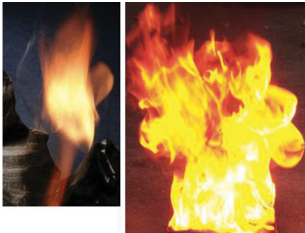
Picture 5.2 images of burning crude oil from shale oil (left) and refined oil (right).
