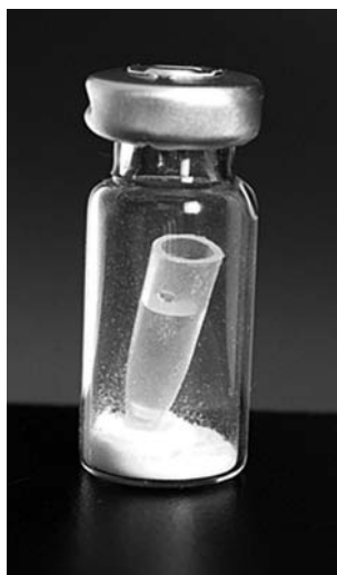
Figure 50 Internal hygostat for microcalorimetry experiments.
