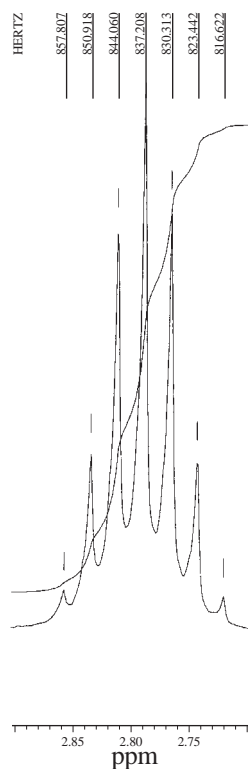
FIGURE 5.28 A septet determined at 300 MHz showing peak positions in ppm and Hz values.
