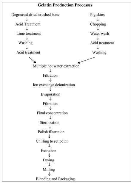
Figure 1: Flow chart for gelatin production process
