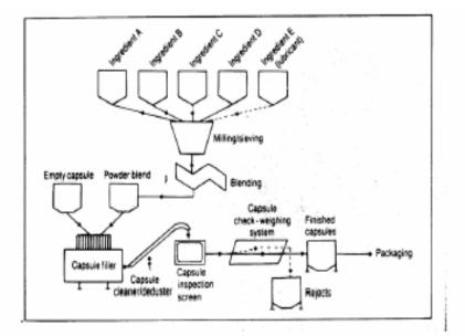
Figure 3: Process flow diagram for automated capsule filling (Source – Textbook of Pharmaceutics by Bentley, 8<sup>th</sup> Edition)
