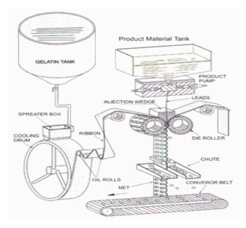
**Figure 8:** Automatic Soft Gelatin Encapsulation Machine (Source - Encycloprdia of Pharmaceutical Technology, Volume – 2)
