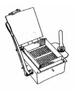
**Figure 2: Hand operated hard gelatin capsule filling machine** (Source: Remington – The Science and Practice of Pharmacy, 20<sup>th</sup> Edition, Volume 1, courtesy – Park Davis)
