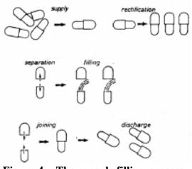
Figure 4: The capsule filling process
