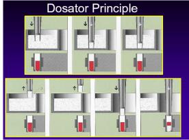
**Figure 5: Dosator principle of filling capsule** (Source - Modern Pharmaceutics by Gilbert S. Bankers, 4<sup>th</sup> Edition, Dekker series)
