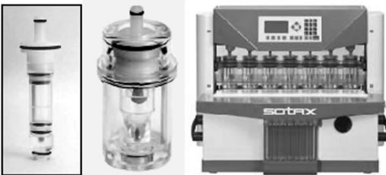
Figure 9 Example of flow-through Apparatus 4 manufactured by Sotax.
