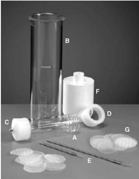
Figure 6 Pictured are various parts of an Apparatus 3: A : internal glass cylinder; B : media vessel; C : end caps for the glass cylinder; D : sampling cannula; E : evaporation cover; F : screens to be placed in the end caps.
