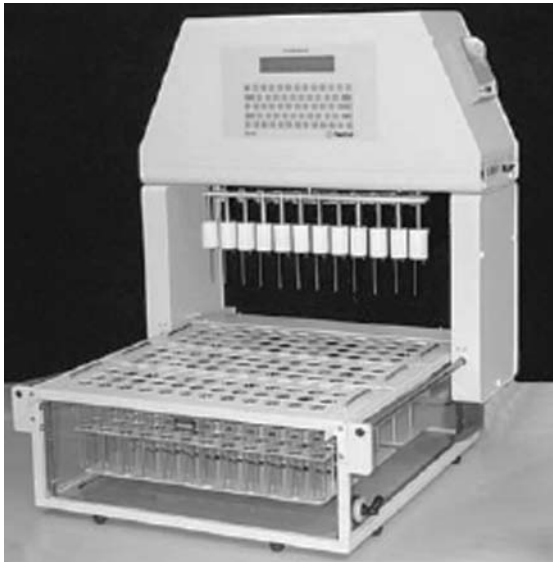
Figure 15 Example of Apparatus 7, with 12 sample locations and 9 rows of tubes. Source: Courtesy of Varian, Inc.
