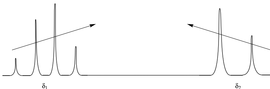
Figure 15.65. The NMR spectrum of a strongly coupled spin system. Note how the inner lines have increased in intensity, and the outer lines have decreased, compared with Fig. 15.62.
