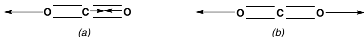
Figure 4.17. The two stretching vibrations of \text{CO}_2 : (a) antisymmetric u and (b) symmetric g .
