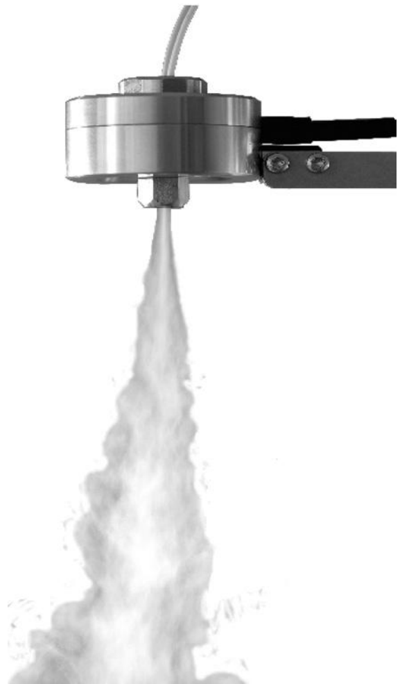
Fig. 29.8 • Two-fluid nozzle atomization. Courtesy of Buchi.
