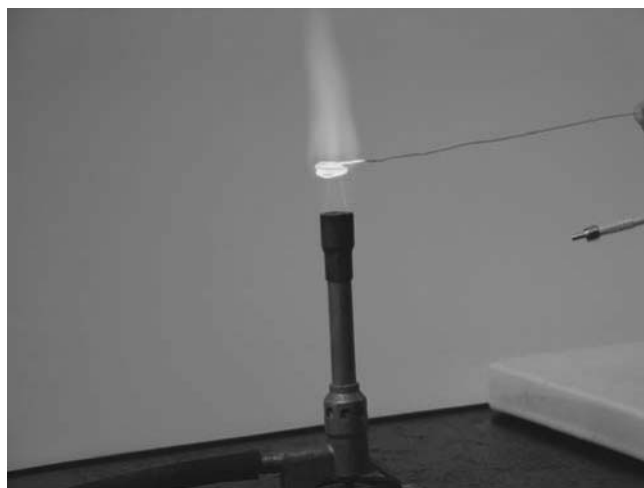
Figure 1 Heating a nichrome wire in the Bunsen burner flame
