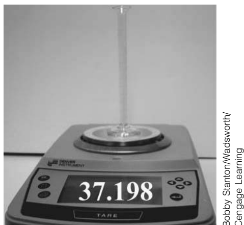
Figure 1 Weighing an empty 10.0 mL graduated cylinder
