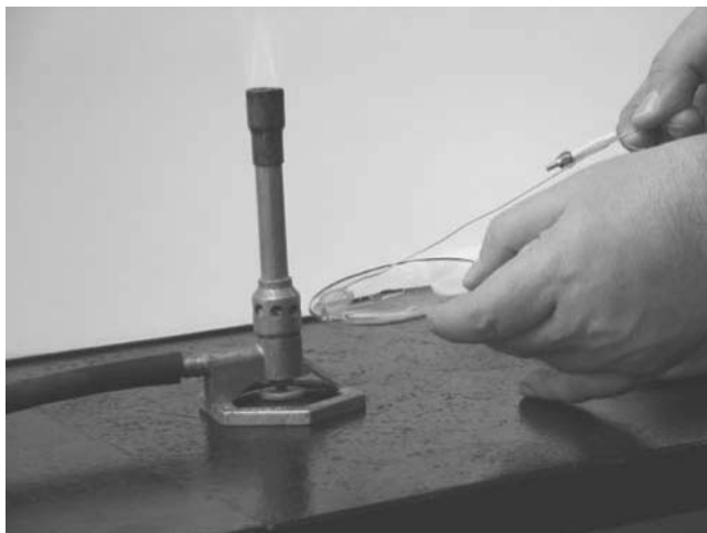
Figure 2 Spattering sample into the Bunsen burner flame
