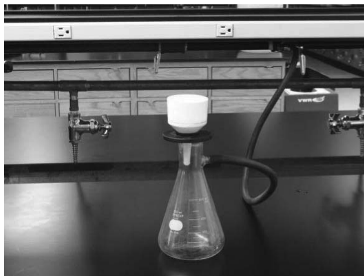
Figure 6 Vacuum filtration apparatus
