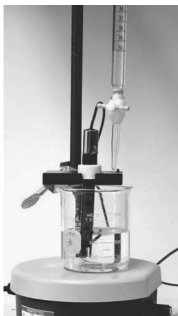
Figure 1 MeasureNet drop counter, pH electrode and buret assembly
