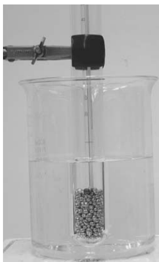
Figure 2 Heating solid inside a test tube immersed in boiling water
