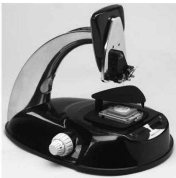
Figure 10.3 A Beecher MTA-2 manual tissue microarrayer (reproduced with permission from Beecher Instruments.)
