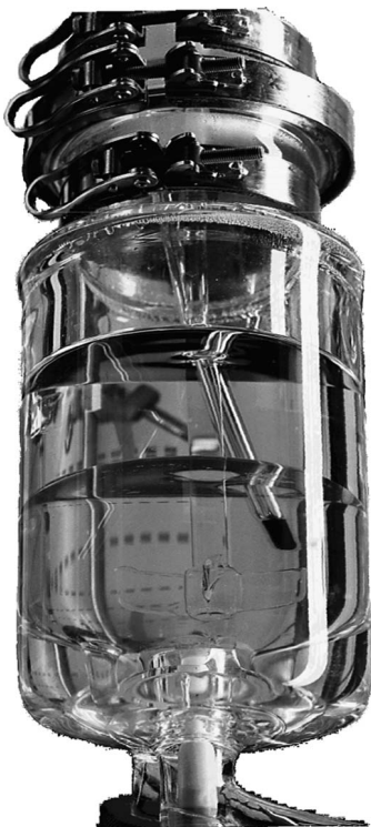
Figure 5.9 The BASIL reactor showing the reaction mixture, the upper phase being the solvent-free pure product, and the lower the ionic liquid. (Photo: BASF.)
