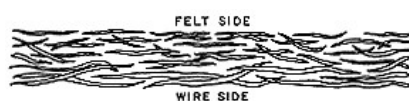
Figure 2.7. Paper and paperboard surface texture is always rougher on the “wire” side than the “felt” side because coarse fibres settle more quickly than finer ones.
