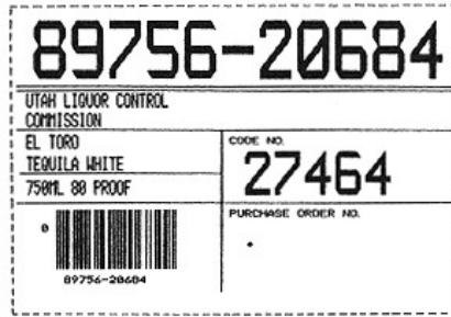
Figure 12.14. Information stored in memory can be used to operate a dot-matrix printer for small quantities of labels. Borders and bar codes are part of the stored data for every product in the line. Purchase order number can be added before printing each batch of labels. (Source: Fleishmann Distilling Corp., used with permission.)
