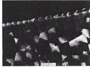
Figure 8.11. Long-chain PE molecules form dendritic (branched) crystals, which are folded back every 100 Å or so, making lamellae that are about 150 layers thick. Chilling of the surface causes spherulites to nucleate very close together. The lamellae, which grow from these nuclei, propagate perpendicular to the surface, since they are restricted by neighboring spherulites. This forms a transcrystalline region, which is about 15 μm (0.0006 in.) thick. (Source: Journal of Applied Physics, used with permission.)
