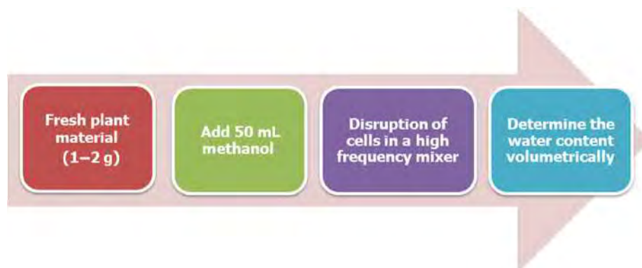
FIG. 4.5 Determination of the moisture content of a fresh crude drug.
