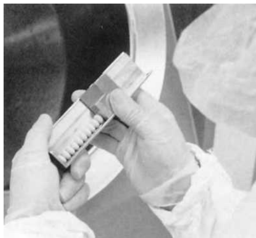
FIGURE 8.32 Gauge used to measure coated tablets. (Courtesy of Eli Lilly and Company.)
