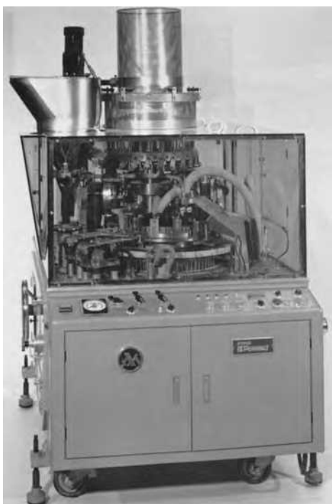
FIGURE 7.10 Osaka Automatic Capsule Filler model R-180, capable of filling up to 165,000 capsules per hour. (Courtesy of Sharples-Stokes Division, Stokes-Merrill, Pennwalt Corporation.)
