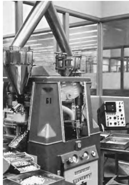
FIGURE 8.25 Manesty Rotapress rotary compression machine. Tablets leaving the machine run over a tablet duster to screen, where they are inspected. Material to be compressed is fed from the overhead hopper through yoke to the two compressing machine hoppers. Hardness of tablet is monitored electronically by oscilloscope at right. (Courtesy of Upjohn Company.)
