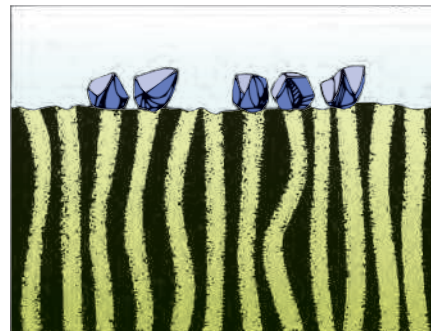
FIGURE 15.4 Membrane filters act as microporous screens that retain all particles and microorganisms larger than the rated pore size on their surface. (Courtesy of Millipore Corporation.)
