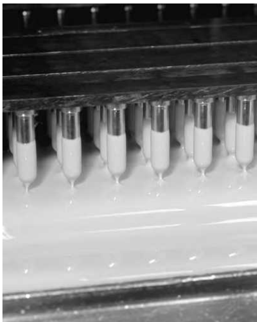
FIGURE 7.3 Capsules being dipped for coloring on automated capsule-making equipment. (Courtesy of Shionogi Qualicaps.)
