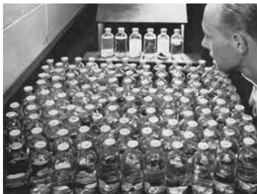
FIGURE 15.12 Testing compatibility of rubber closures with a solution. (Courtesy of Abbott Laboratories.)
