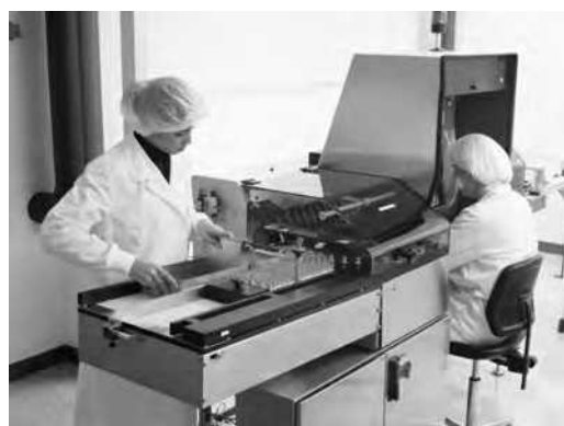
FIGURE 15.24 Semiautomatic inspection machine for parenteral products. (Reproduced with permission of Schering Corporation. All Rights reserved.)
