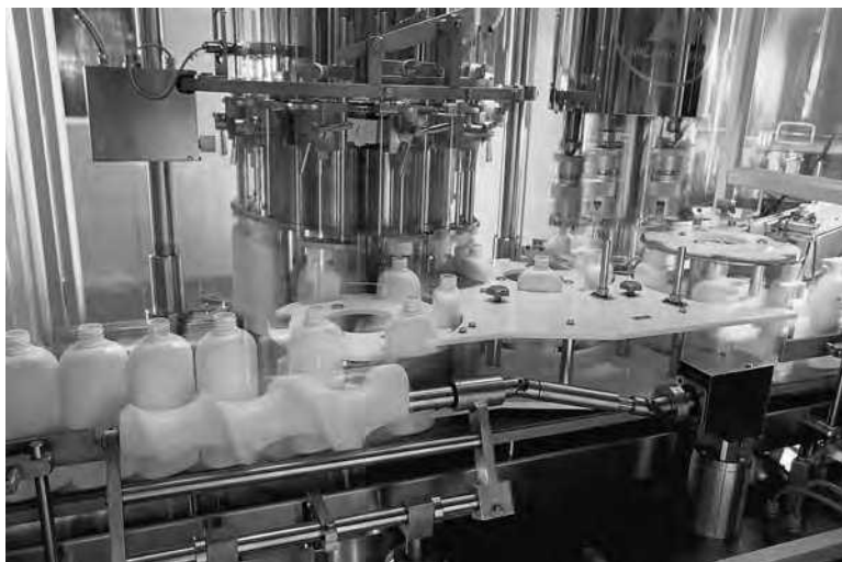
FIGURE 14.6 Liquid filling. Bottles being conveyed after cleaning. As they pass through an indexing worm, the bottles are spaced accurately for filling and capping. (Courtesy of Paddock Laboratories.)
