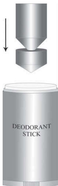
Figure 3.34 Hardness testing of a deodorant/antiperspirant stick. Adapted from Texture Technologies Corp.
