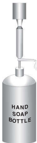
Figure 3.11 Actuation force testing of a pump-head container. Adapted from Texture Technologies Corp.
