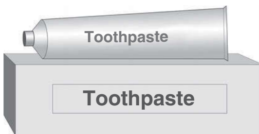
Figure 2.2 A cosmetic package, including an outer container (i.e., a folding carton) and an immediate container (i.e., a plastic tube).
