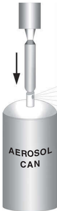
Figure 3.27 Actuation force testing of an aerosol can.
