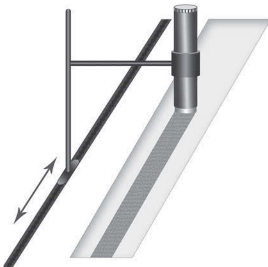
Figure 3.30 Payoff and glide testing of a sunscreen stick. Adapted from Texture Technologies Corp.
