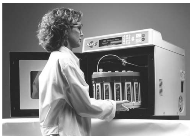
Figure 1.6 A commercial analytical microwave digestion system for sealed vessel digestion of multiple samples. Courtesy of CEM Corporation, Matthews, NC ( www.cem.com ).
