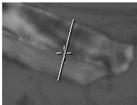
Figure 4.25 Micrograph of a polymer laminate, showing two broad layers and a narrow middle layer. The sample was mounted in an NaCl compression cell and spectra were collected automatically in 2\ \mu\text{m} steps along the white line indicated. A Centaurus Analytical FTIR Microscope System from ThermoNicolet was used for the automatic data collection and results presented in this figure and in Figs. 4.26–4.28. [Courtesy of ThermoNicolet, Madison, WI ( www.thermonicolet.com ).]
