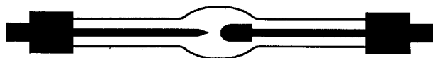
Figure 5.42 Compact xenon arc lamp used in fluorometers. The quartz envelope is filled with xenon gas. The lamp is ignited by a 10–20 kV pulse across the electrodes. (From Froelich and Guilbault, used with permission.)
