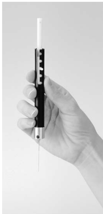
Figure 1.11 An SPME probe the size of a ballpoint pen. Reprinted with permission of Supelco, Bellefonte, PA 16823, USA ( www.sigma-aldrich.com ).
