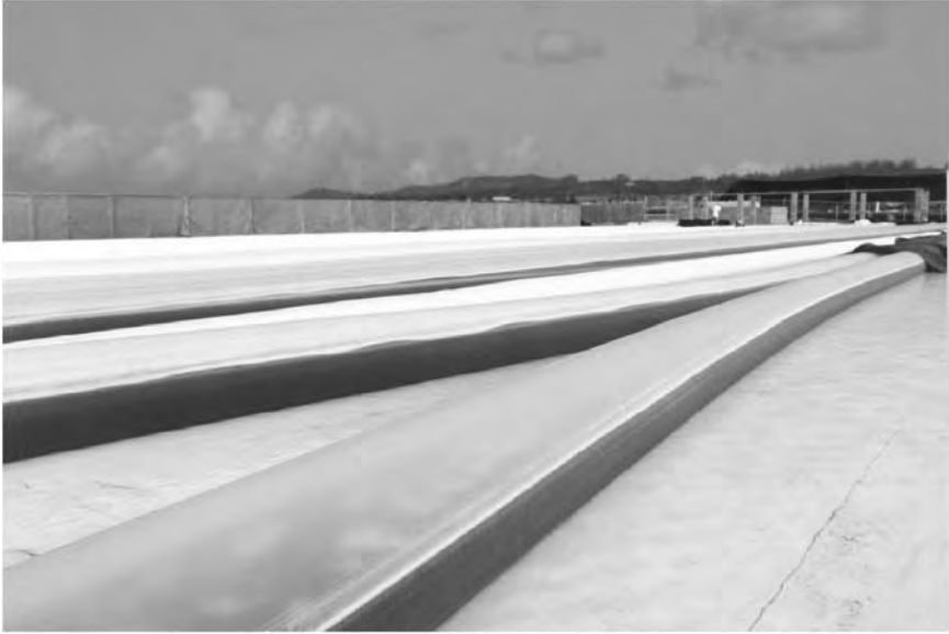
FIGURE 13.4 The Mera growth module, an enclosed photobioreactor used for the production of Haematococcus pluvialis biomass.
