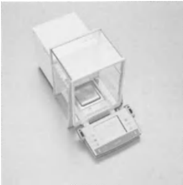
Figure 2. Analytical balance Mettler AX201. 220 \text{ g} \times 0.01 \text{ mg} Automatic self-calibration with built-in reference masses.
