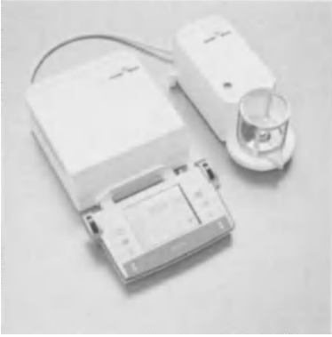
Figure 1. Microbalance Mettler MX5. 5100 \text{ mg} \times 1 \mu\text{g} Automatic self-calibration with built-in reference masses.
