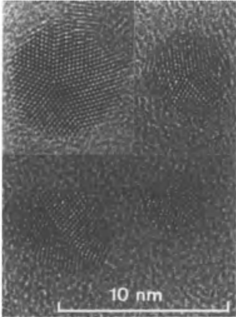
Figure 70. Small silver particles consisting of an icosahedral aggregate of multiply twinned face-centered cubic crystals (Courtesy of C. Goossens)
