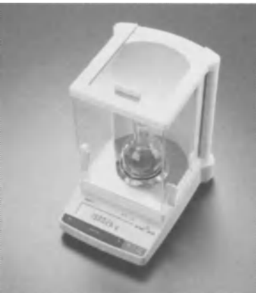
Figure 3. Analytical balance Mettler AB204-S. 210 \text{ g} \times 0.1 \text{ mg} Self-calibration with built-in reference mass.
