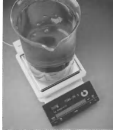
Figure 4. Precision balance Mettler PR8002, DeltaRange, 8100 \text{ g} \times 0.01 \text{ g} Self-calibration with built-in reference mass.
