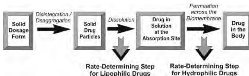
Fig. 2.15. The two rate-determining steps in the absorption of drugs from orally administered formulations
