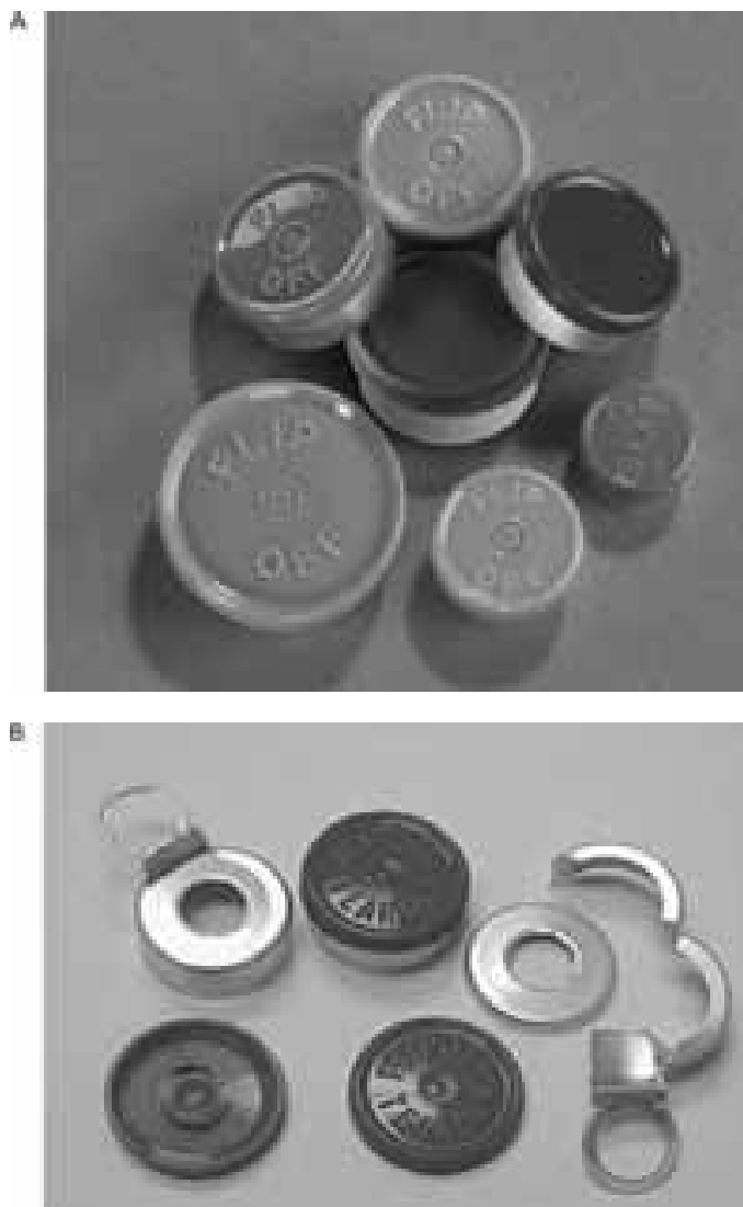
Figure 26-25. Examples of aluminum-plastic seals. A. Flip-Off Seals: Aluminum shell with a removable plastic button in order to access stopper surface. B. Flip-Tear Seals: Aluminum shell is completely removed from container by flipping off the plastic button—allows stopper removal. (Courtesy of West Pharmaceutical Services.) (Flip-Off is a registered trademark of West Pharmaceutical Services in the United States and other jurisdictions.)
