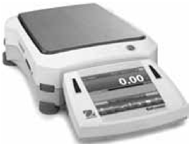
Figure 9-4. Electronic single-pan balance. (Courtesy of OHAUS Corporation.)
