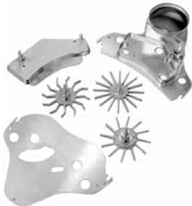
Figure 30-20. Forced Flow Feeder. (Courtesy of Fette.)
