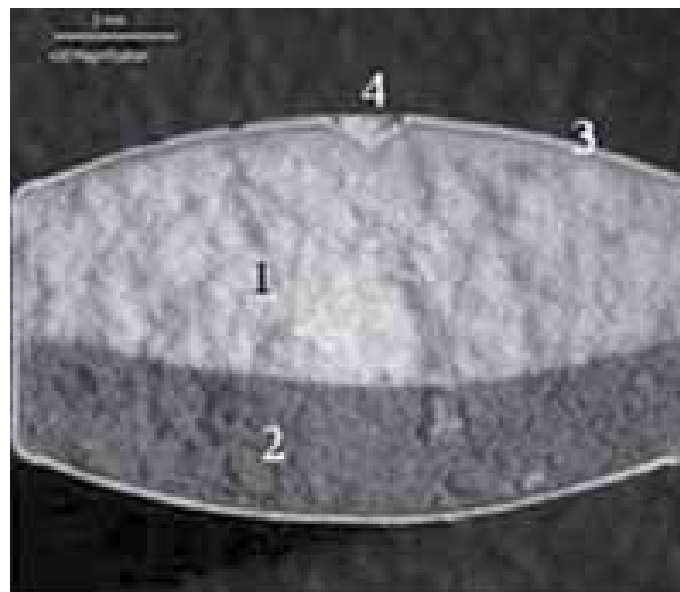
Figure 32-8. Cross-section of a push–pull osmotic pump (PPOP) tablet. 1. Pull layer (drug layer). 2. push layer, 3. semipermeable membrane, 4. drug delivery orifice.
