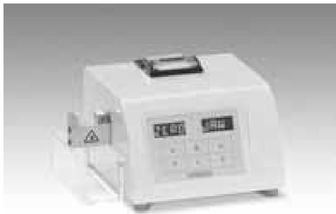
Figure 30-29. Electric Tablet Hardness Tester. (Courtesy of Erweka.)
