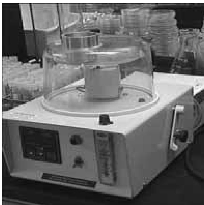
Figure 26-14. Examples of a Slit-To-Agar (STA) Quantitative Air Sampler.
