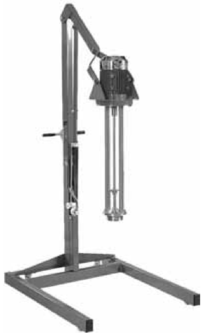
Figure 24-5. Pilot Scale Rotor Stator. (Courtesy of Silverson Machines, Ltd.)
