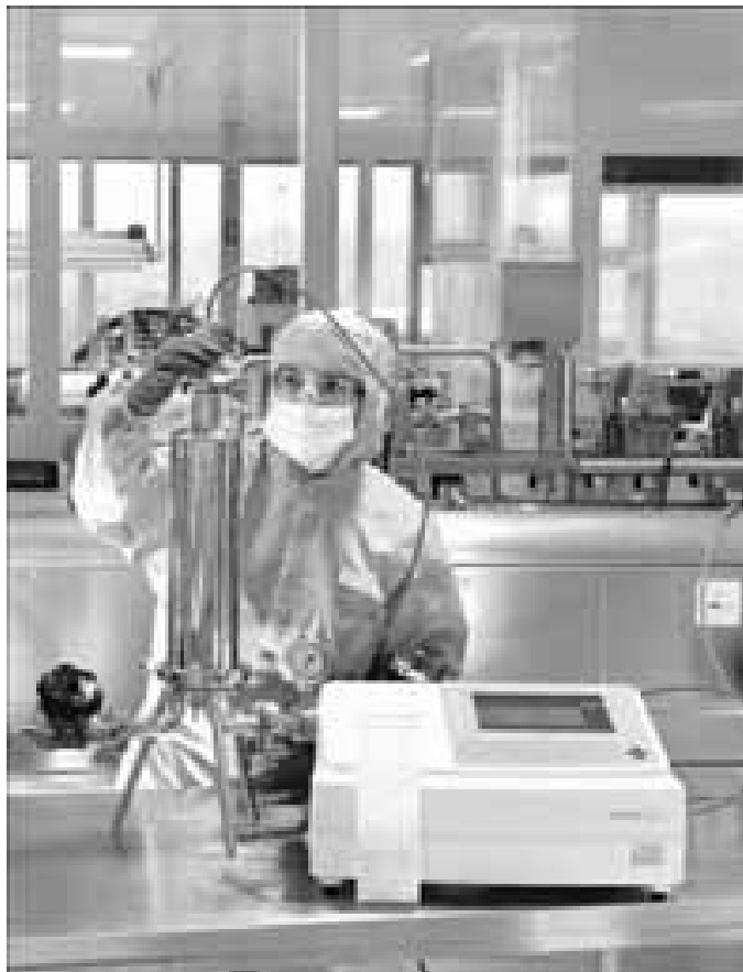
Figure 25-22. Performing an automated integrity test on a cartridge filter. Courtesy of Sartorius Stedim Biotech.
