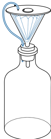
Figure 14-7. Filtration of volatile liquids.
