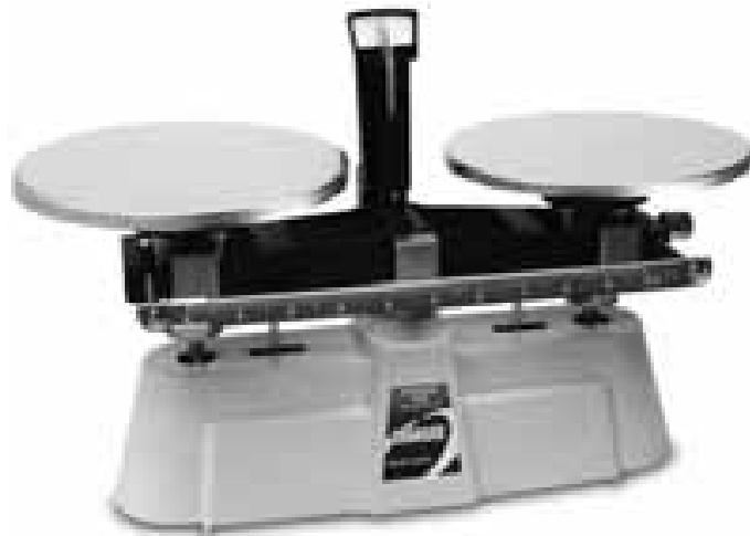
Figure 9-2. Single-beam equal-arm balance. (Courtesy of OHAUS Corporation.)
