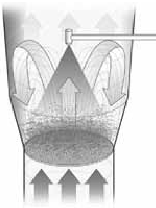
Figure 30-13. Fluid Bed Top Spray Granulator. (Courtesy of Glatt.)
