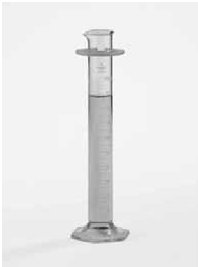
Figure 9-8. Glass cylindrical graduate. (Courtesy of Kimble Glass.)
