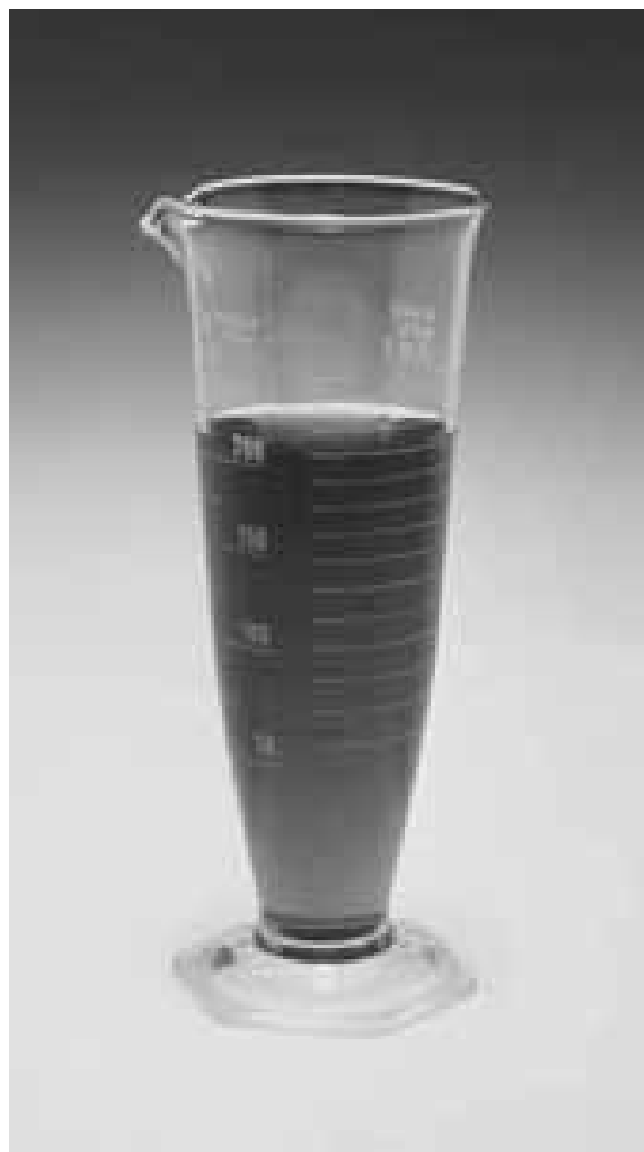
Figure 9-7. Class conical graduate. (Courtesy of Kimble Glass.)
