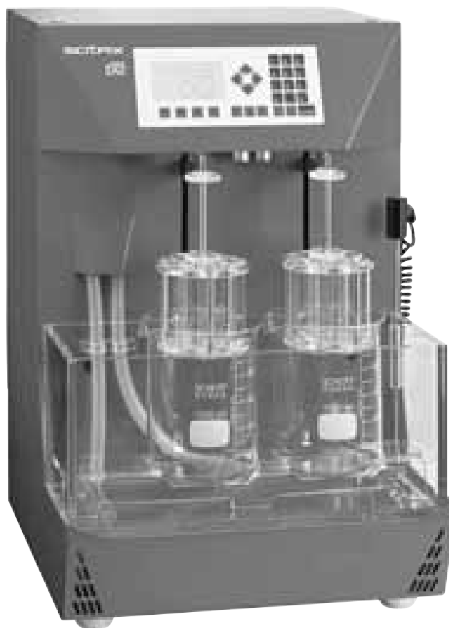
Figure 30-33. USP Disintegration Tester. (Courtesy of SOTAX.)
