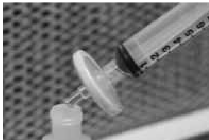
Figure 14-3. Example of a filter membranand holder (Luer lock syringe membrane filter). (Courtesy of PCCA-Professional Compounding Centers of America.)
