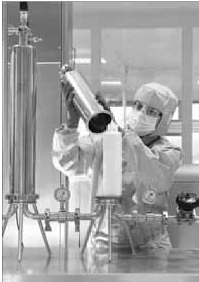
Figure 25-20. Assembling a cartridge filter and its housing. Courtesy of Sartorius Stedim Biotech.
