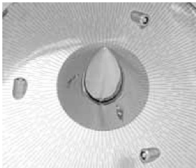
Figure 30-17. Disk Jet. (Courtesy of Hüttlin GmbH, A Bosch Packaging Technology Company.)
