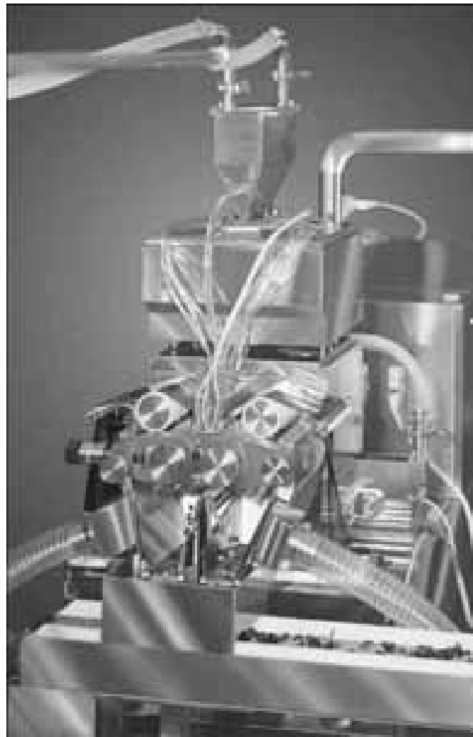
Figure 30-45. Rotary-die soft gelatin capsule filler. (Courtesy of Pharmagel Engineering SPA: Milan, Italy.)
