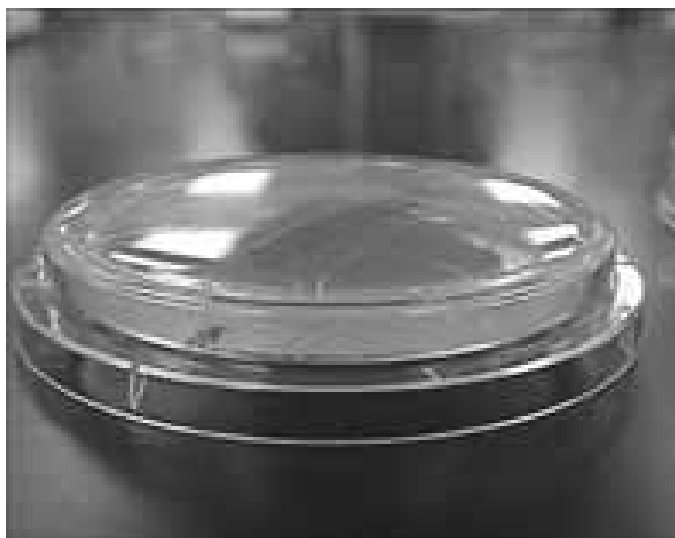
Figure 26-15. Example of a Rodac plate. (Courtesy of Baxter Healthcare Corporation.)
