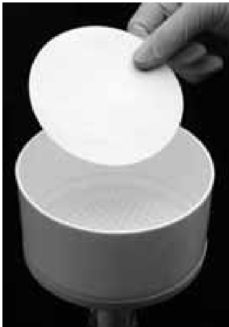
Figure 14-2. Example of filter paper used in laboratory filtrations. (Courtesy of PCCA-Professional Compounding Centers of America.)
